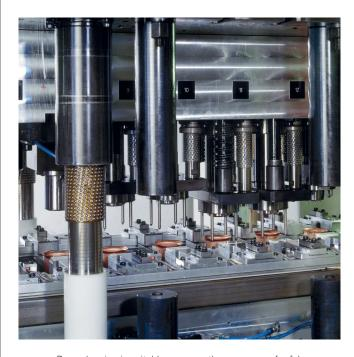
Deep drawing is suitable, among other purposes, for fabricating hollow bodies with a wall thickness ranging from 0.1 to 2 mm. After the blanks are cut, the workpieces are brought into their final shape, undergoing as many as 22 different forming and shaping operations in the process.
