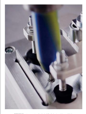
GESIPA® set new standards in blind rivet setting with its latest innovation, the new FDR® (Flow Drilling Rivet®). It combines the drilling of the rivet hole and the riveting itself in a single step, resulting in significant efficiency
